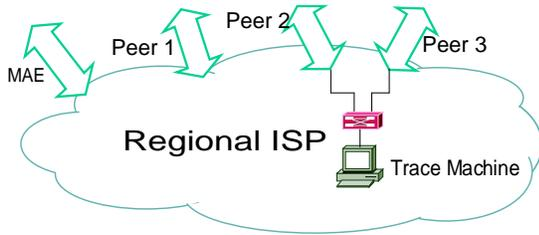
**Figure 4: The trace machine monitors two of the four peering links at Los Nettos.**
